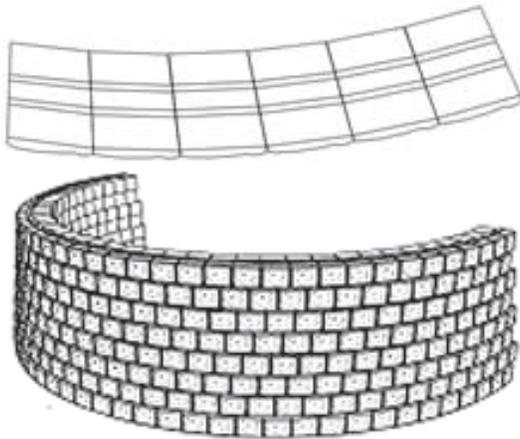
Taper units are used to construct outside curves. For smooth flowing curves, place all units tapered on the left side on one course, and all units tapered on the right side on the next course.
