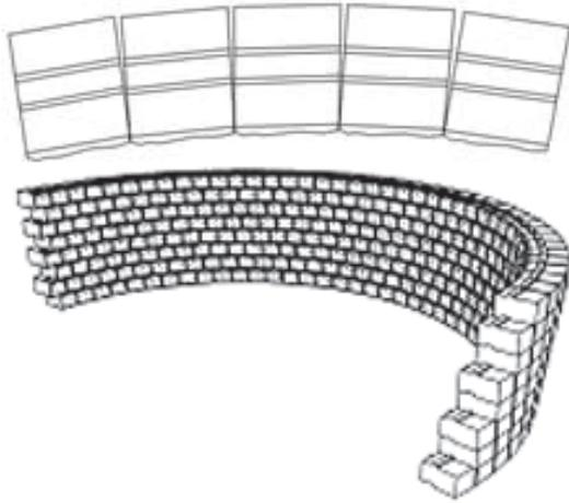
Standard units are typically used to construct inside curves. The front faces of the units are placed tightly together while small spaces are left between the back of the units.
